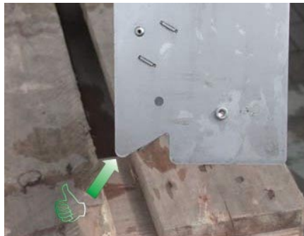
14) Correct: Screen is aligned with triangular cutout .
