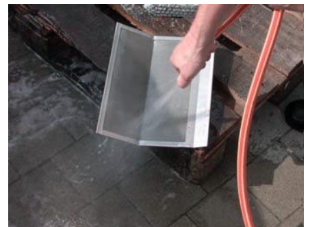
9) Finally rinse off the screen with a strong water jet.
