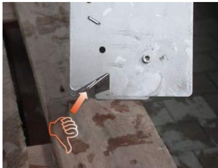
13) Double-check the correct seat of the filter: The screen shall not be visible in the triangle indicated in the picture.
