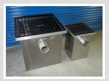
Inlet sump/sand trap 300/600 is the first stage of the oil separation process. Installed upstream (before) grit trap and oil separator. It is designed to collect and catch solids with a specific gravity of over 1. The inlet sump has a removable Basket and mentis grate cover with a 100mm ID outlet connection. To clean sump, remove basket with accumulated solids and discard accordingly.
